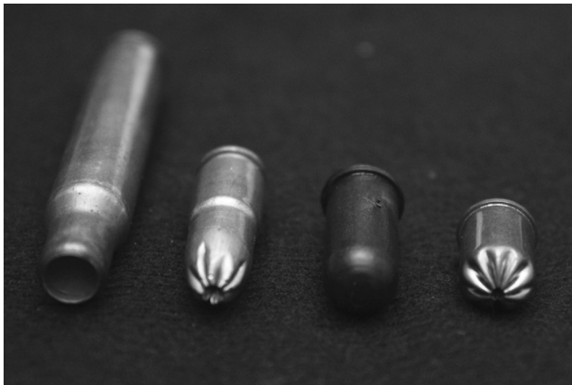
Figure 2.29 An assortment of blank cartridge styles. Some have “rosette” or crimped necks, while others use a cap to cover the interior. (Image from author's collection.)
